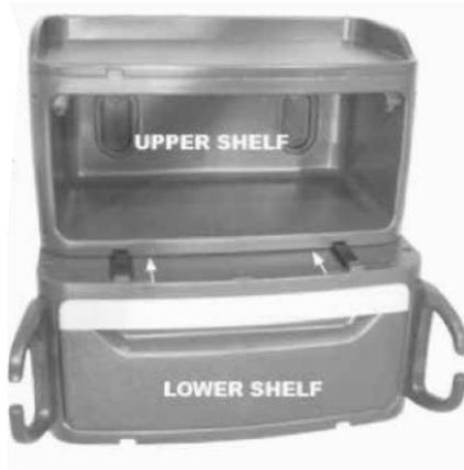
3. With the unit lying flat, locate the wide slot at the bottom of the spine. 4. Place the connected shelves into the slot and slide in and up the spine. The lower shelf with side handles should be closest to the base.
